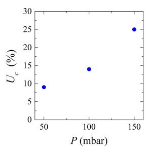
**Figure 5.** Percentage of unstable clogs  $(U_c)$  for different system pressures (P).
