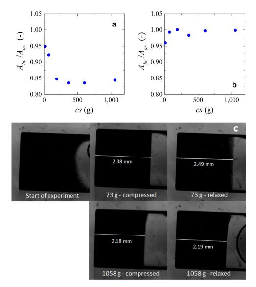
**Figure 8.** (a) Compression data of microgels. Ratio between area after compression ( $A_{ac}$ ) and the area before compression ( $A_{bc}$ ) versus centrifugation speed (cs). (b) Relaxation data of microgels. Ratio between area after ( $A_{ar}$ ) and before relaxation ( $A_{br}$ ) versus centrifugation speed (cs). (c) images showing the compressed and relaxed microgels at low and high number of g-forces. Values of area were measured manually with an average measurement error <0.5%.
