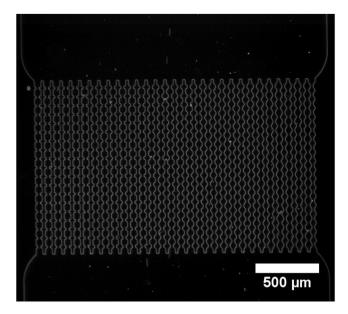
**Figure 1.** Optical microscopy image of the array of channels that compose the microfluid device at 2.5x magnification. There are 30 parallel channels with five different entrance angles. From left to right: 0°, 20°, 35°, 45°, 55° (see Fig. 2a).
