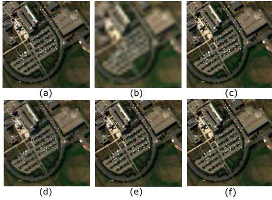
Fig. 11. Fusion results (Pavia Data Set). (a) MS image. (b) HS image. (c) FUMI method with no compression. (d) Method proposed in [20] using C-CASSI. (e) Proposed method with 50% compression using C-CASSI. (f) Proposed method with 50% compression using SSCSI.
