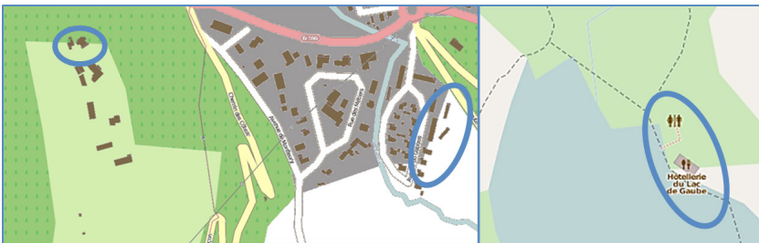
Fig. 1: Examples of LoD inconsistency in OSM. On the left, the rough built-up areas/forest limits intersect detailed buildings; on the right, detailed footpaths lie on the surface of a roughly digitised lake. ©OpenStreetMap contributors.
