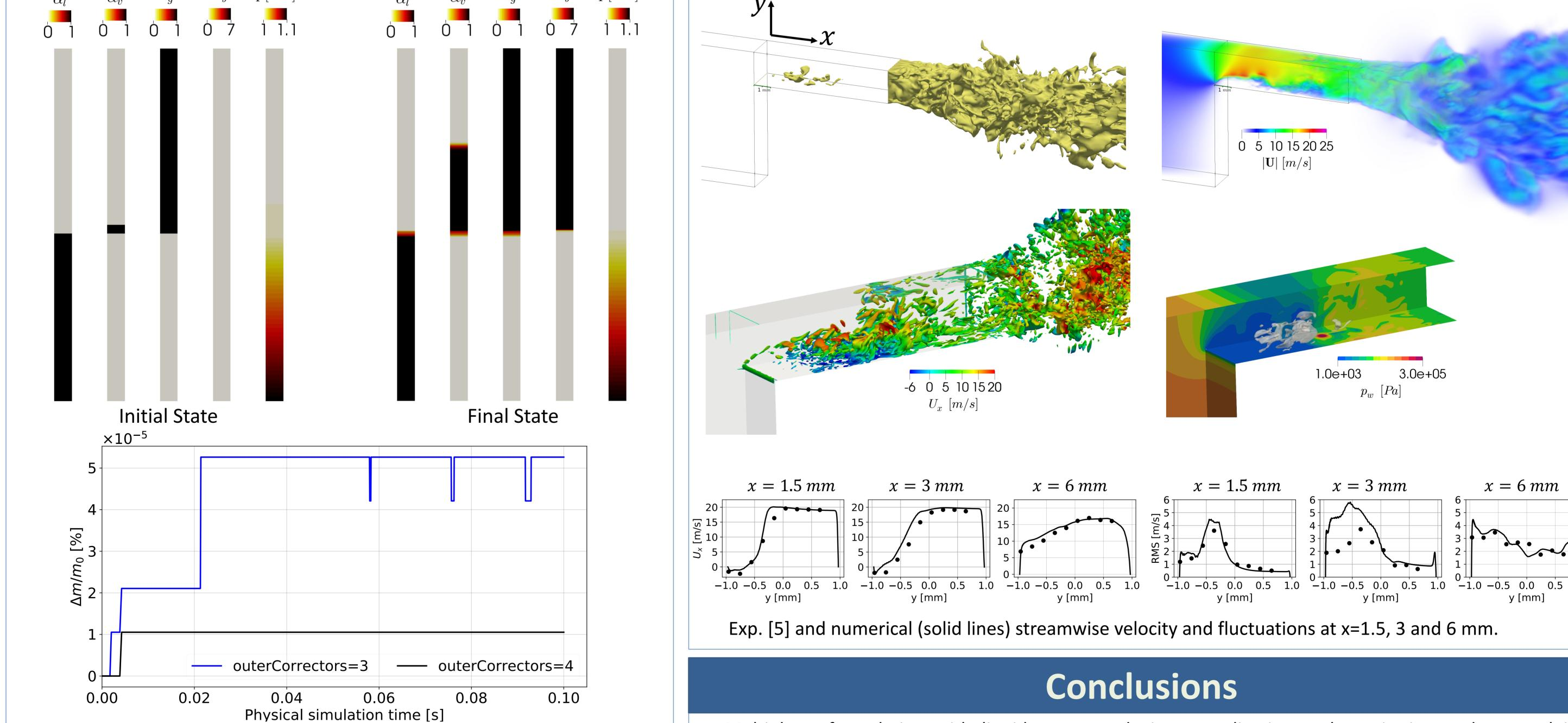
A column of liquid and gas (air and vapor) is set with hydrostatic pressure distribution initially (top right). After the onset of cavitation, the total mass of liquid and vapor is compared (bottom), as the liquid changes to vapor (top left). Mass is conserved with good accuracy.
