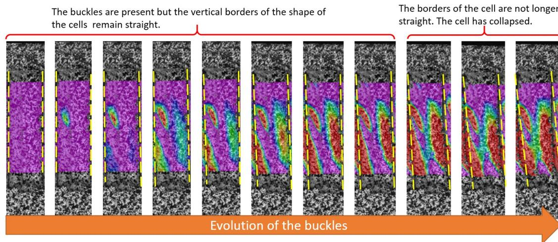
Figure 8: Buckling evolution of a cell
