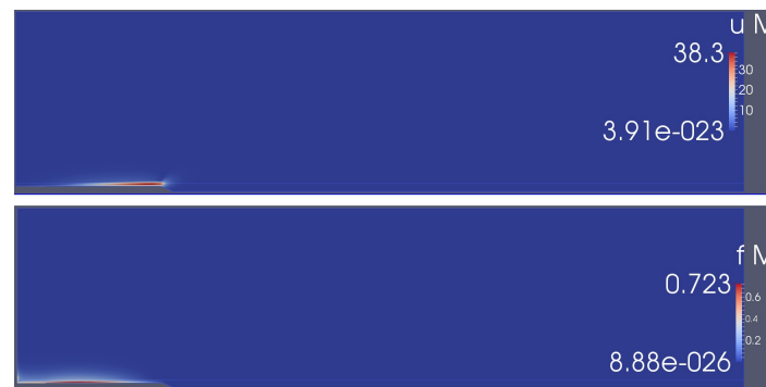
Figure 11. Magnitude of the sub-optimal (penalized) response and forcing fields, |u''| and |f| , in the upper and lower panels, respectively, at \text{Re} = 1000 and \beta = 1 . The gain is maximized following (11).
