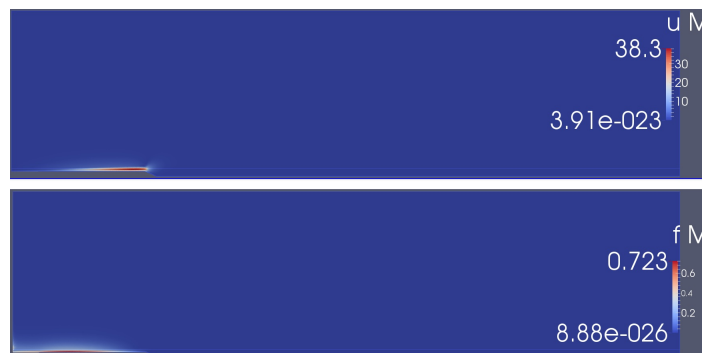
Figure 11. Magnitude of the sub-optimal (penalized) response and forcing fields, |u''| and |f| , in the upper and lower panels, respectively, at Re = 1000 and \beta = 1 . The gain is maximized following (11).
