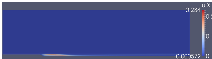
Figure 9. Horizontal component u'' of the dominant perturbation field at Re = 1000 and \beta = 1 .
