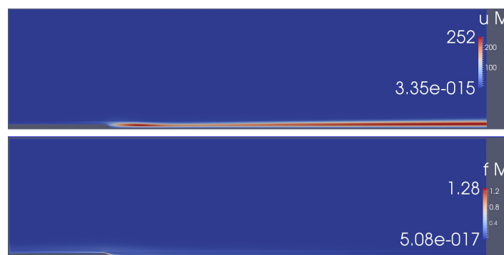
Figure 10. Magnitude of the optimal response and of the corresponding optimal forcing fields, |u''| and |f| , in the upper and lower panels, respectively, at Re = 1000 and \beta = 1 . The gain is maximized according to (7).
