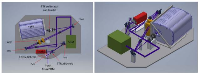
Figure 10. Preliminary mechanical layout of LNGS sensors.
