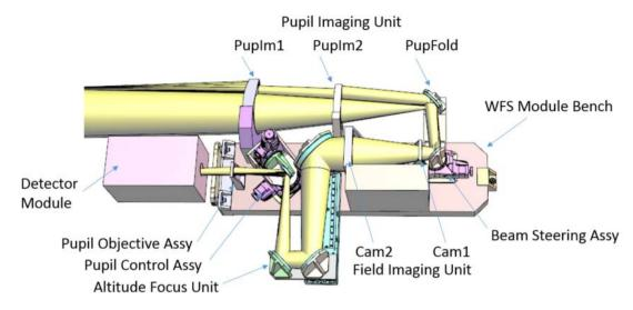
Figure 8. Opto-mechanical design of the LGSS wavefront sensor module.
