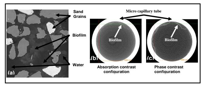
**Figure 1:** (a) Image (1.8mm x 2 mm) showing sand grains, biofilm containing inorganic matter and water. This image is obtained with the absorption contrast configuration. Biofilm with water in micro capillary tube (of 2 mm outer diameter) with (b) absorption contrast configuration and (c) phase contrast configuration. The voxel size for these images is  $2.5 \, \mu m$ .
