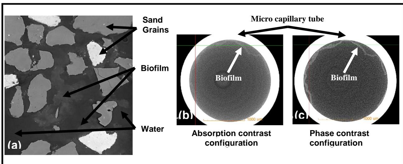
**Figure 1:** (a) Image (1.8mm x 2 mm) showing sand grains, biofilm containing inorganic matter and water. This image is obtained with the absorption contrast configuration. Biofilm with water in micro capillary tube (of 2 mm outer diameter) with (b) absorption contrast configuration and (c) phase contrast configuration. The voxel size for these images is 2.5 µm.
