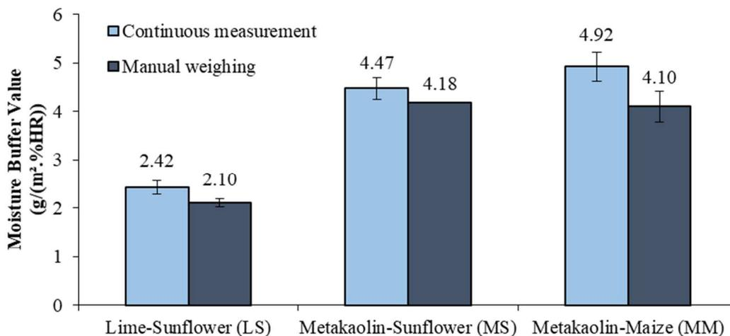
Figure 14 - Moisture buffer values of vegetal concretes.
