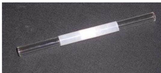
Fig. 5. Picture of a cladded MonoSil-SOD (0.6 x 1 cm) with glass connections.
