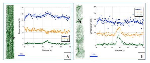
Figure 1 Reconstructed analyzed volumes of (a) annealed UFG sample and (b) irradiated UFG sample showing distribution of Si. Line profiles of elemental distribution across grain boundaries as indicated for Si, Cr and Ni.
