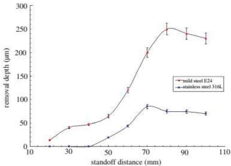
Figure 8: Removal depth (µm) versus standoff distance (mm) for E24 and 316L steels (operating pressure is 210 MPa). (Online version in colour)
