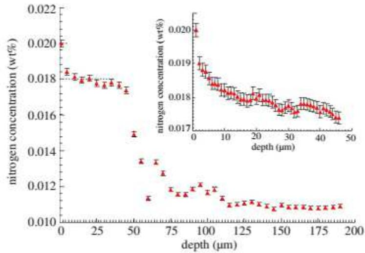
Figure 14: Profile of nitrogen concentrated (wt%) versus depth ( $\mu\text{m}$ ) in mild steel E24 on 200  $\mu\text{m}$  of depth below the crater. Inset: Profile on 50  $\mu\text{m}$  of depth below the crater. Error bars are added. (Online version in colour)
