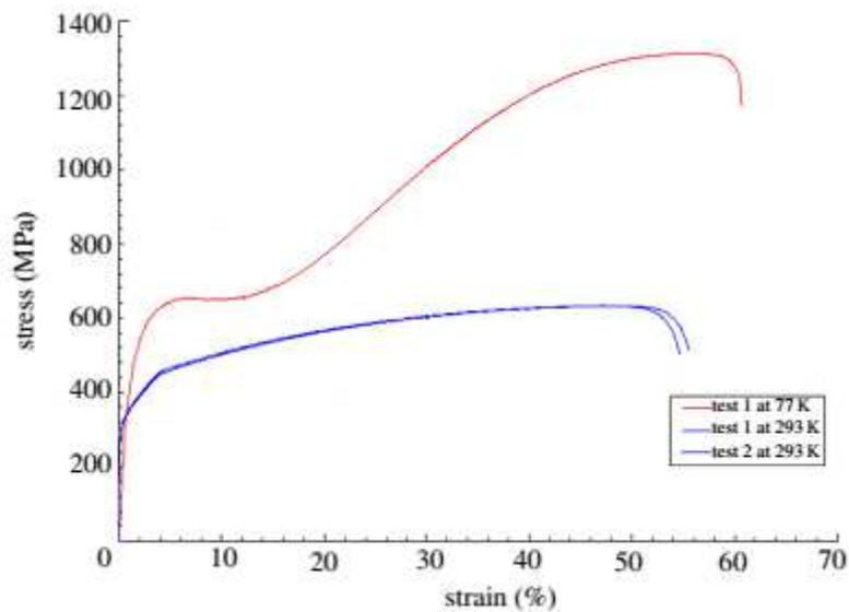
Figure 4: Stress versus strain curves of fcc stainless steel 316L at low and room temperatures. (Online version in colour)
