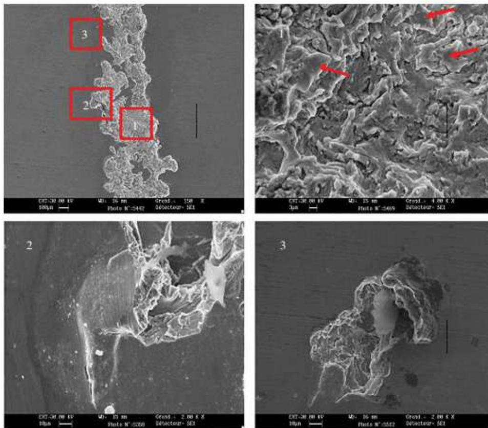
Figure 9: Typical damage identified for 316L steel (for all standoff distance in the range 50-90 mm). Blow-ups in insets: (1) brittle fracture; (2) lifting of a chip at the edge of the groove; and (3) spalling. (Online version in colour)
