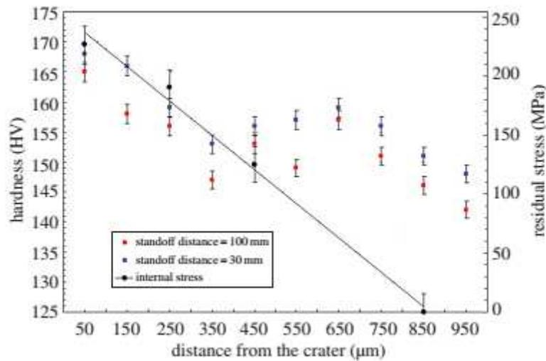
Figure 11: Hardness and internal stress versus distance from groove in mild steel E24. The sign of internal stress was changed for convenience (they are compressive stresses). Errors bars are added. (Online version in colour)
