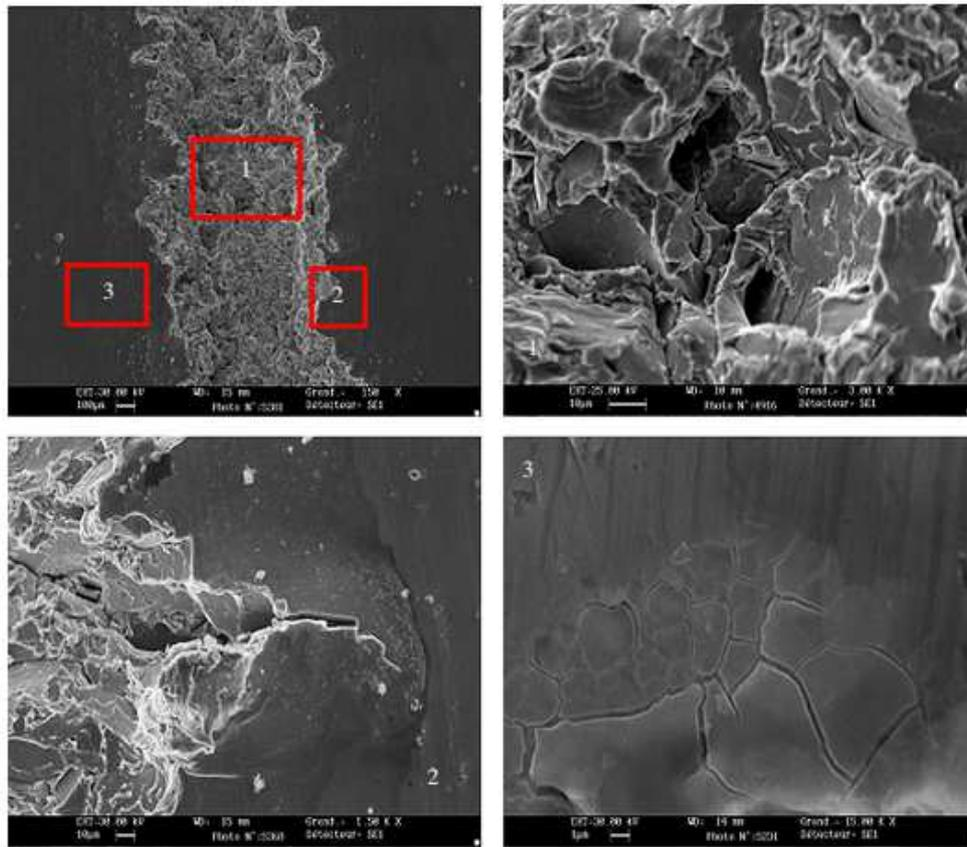
Figure 10: Typical damage identified in mild steel E24 (for all standoff distance in the range 50-100 mm). Blow-ups in insets: (1) intergranular fracture by cleavage; (2) cracking at the crater's edge and (3) interconnected network of microcracks. (Online version in colour)
