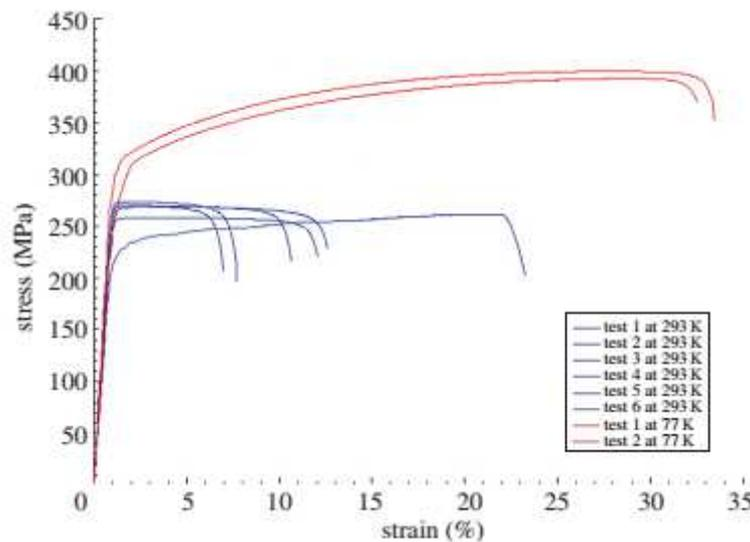
Figure 2: Stress versus strain curves of OFHC copper at low and room temperatures. (Online version in colour)
