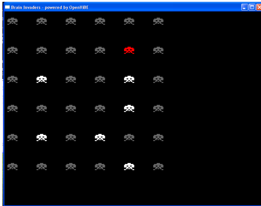
Figure 3. Interface of Brain Invaders during the first level at the moment where a group of six non-Target symbols flash (in white). The red symbol is the Target. The non-Targets which are not flashing are in grey.
