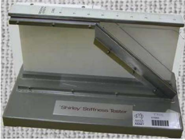
Fig. 6. Standard cantilever bending test with an inclined plane at 41.5°.
