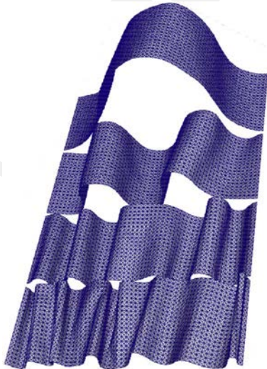
Fig. 14. Wrinkling in compression of a woven reinforcement strip with different bending stiffnesses (from bottom to top 1, 10, 10^2 , 10^3 N/mm).
