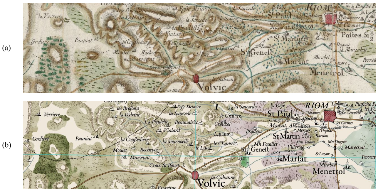
Fig. 2 (a) a view on the original Cassini map of France (sheet 52, 1759-1777) and (b) the extracted vector data mapped with the "Cassini" map style (2019).
