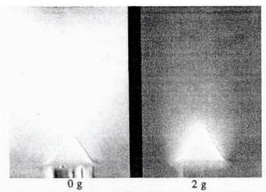
Flow rate of methane 0.22 l/m; flow rate air 1.75 l/m; richness 1.20; pressure 0.9 atmosphere.
