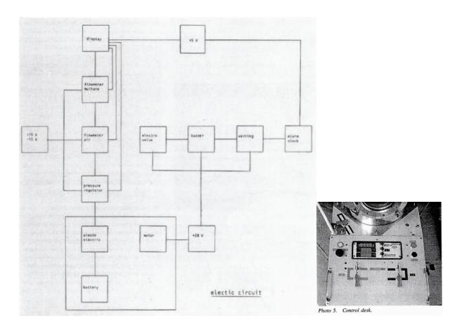
Figure 5. Synoptic sketch of the electric circuit.
