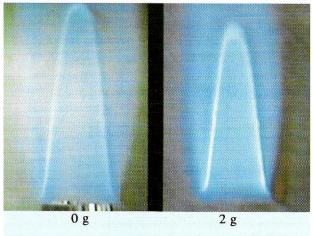
Flow rate of methane 0.33 l/m; flow rate air 2 l/m; richness 1.57; pressure 1 atmosphere.
