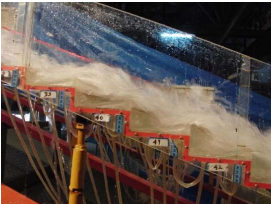
Fig. 13. 12 degrees slope and 30 liter per second flow rate
