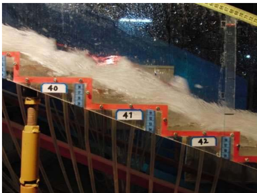
Fig. 6. Horizontal steps with flow rate of 30 liters per second
