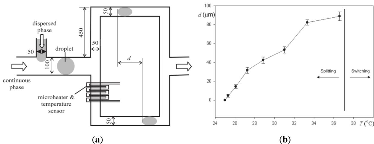
Another 1D droplet handling can be performed using the integration of a serpentine-like micro-heater which locally generates a temperature gradient together with a local decrease in the continuous phase
