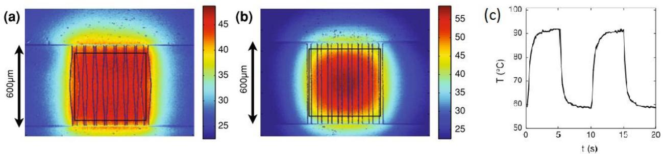
**Figure 15.** Temperature in the working channel as a function of the squared input voltage. The three insets are IR images illustrating the spatial distribution. Reprinted with permission from [67]. Copyright 2009, American Institute of Physics.
