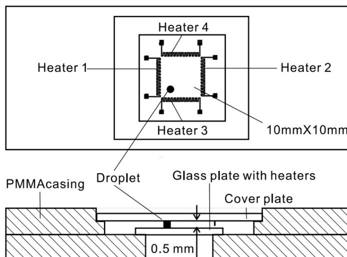
In such a configuration, it is possible to drive droplets by imposing a succession of different temperature gradients along the 2D substrate. The four microheaters actuated independently generate variable surface tension gradients. The droplet can be positioned anywhere in the channel depending on the strength of individual heaters (Figure 18).
