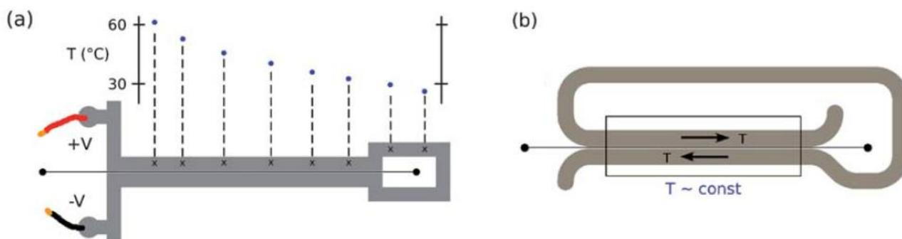
This technique can be combined with the pre-heated liquid technique as reported by Vigolo *et al.* [79] for thermophoresis studies (see Section 5). The authors describe a method for selective driving of particles towards either the hot or the cold side by adding specific electrolytes to their initial solution. The authors used a microfluidic device where temperature gradients were established by combining
