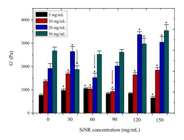
**Fig. 3** Storage modulus (G') of SiNR-collagen composite hydrogels with various collagen and silica concentrations. Variance of the G' value between the hydrogels with same collagen concentration was determined
