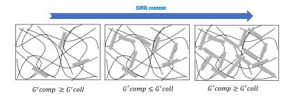
**Fig. 8** Schematic evolution of elastic modulus of composite hydrogels with nanorods concentration at fixed collagen content.
