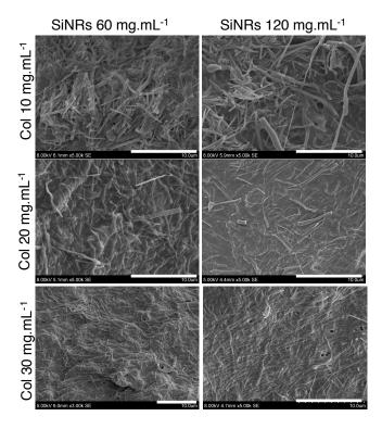
Fig. 2 Selected SEM images of SiNRs-collagen nanocomposites at collagen concentrations 10, 20 and 30 mg.mL
