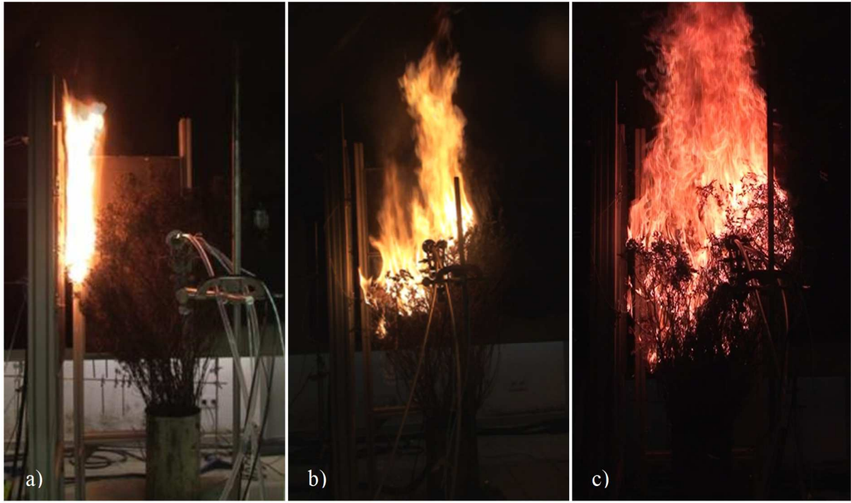
Fig. 6. Fire growth observed 30 s after ignition for different values of \alpha : (a) low combustibility: \alpha = 0.10 \text{ kW}\cdot\text{s}^{-2} (fire test 4); (b) medium combustibility: \alpha = 0.22 \text{ kW}\cdot\text{s}^{-2} (fire test 14) and (c) high combustibility: \alpha = 0.52 \text{ kW}\cdot\text{s}^{-2} (fire test 15)
