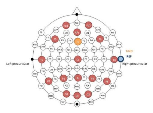
**Figure 1.** The 16 electrodes placed according to the 10-10 international system. In yellow: Ground (GRN) FZ. In blue: Reference (REF) left earlobe.
