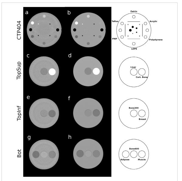
**Figure 2.** Reconstructed experimental pCT and DECT images. The left column contains images reconstructed from experimental pCT data and the middle column from measured DECT data. An RSP level of 1.0 and window of 1.5 were applied on the images for display purposes. The right column contains drawings of the phantoms with the insert materials labeled.
