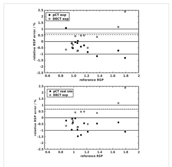
$\label{eq:Figure 3.} Figure 3. \ The RSP \ accuracy \ as \ a function of the reference RSP \ from \ (top) \ experimental \ pCT \ and \ (bottom) \ realistically \ simulated \ pCT \ is indicated \ with \ open \ square \ markers. \ The \ dashed \ and \ dotted \ horizontal \ lines \ indicate \ the \ MAPE \ for \ pCT \ and \ DECT, \ respectively.$
