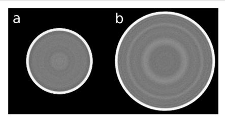
**Figure 6.** pCT images from realistic simulation processed with the *SimCalib2* calibration and tracker gaps filled with silicon. In (a) the 150.5 mm diameter water phantom and in (b) the 225.75 mm diameter water phantom. An RSP level of 1.0 and window of 0.3 were applied on the images for display purposes.
