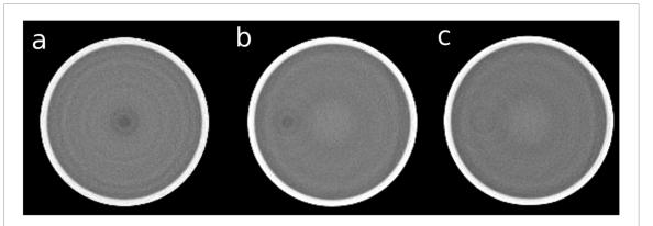
**Figure 5.** pCT images from realistic simulations processed with the SimCalib2 calibration. In (a), the water phantom was aligned to the isocenter, while in (b) and (c) it was shifted by 40 mm with respect to the isocenter. In (a) and (b) the tracker layer gaps were filled with air. In (c), the tracker layer gaps were filled with silicon. An RSP level of 1.0 and window of 0.3 were applied on the images for display purposes.
