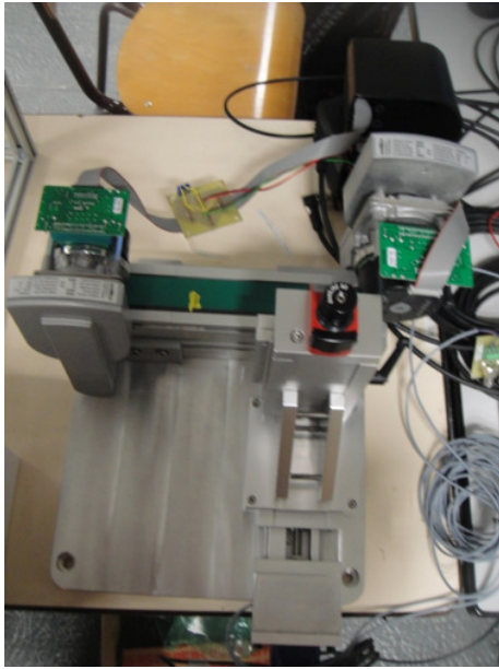
Fig. 5. X-Y table to ensure the rotation of the guide wire
