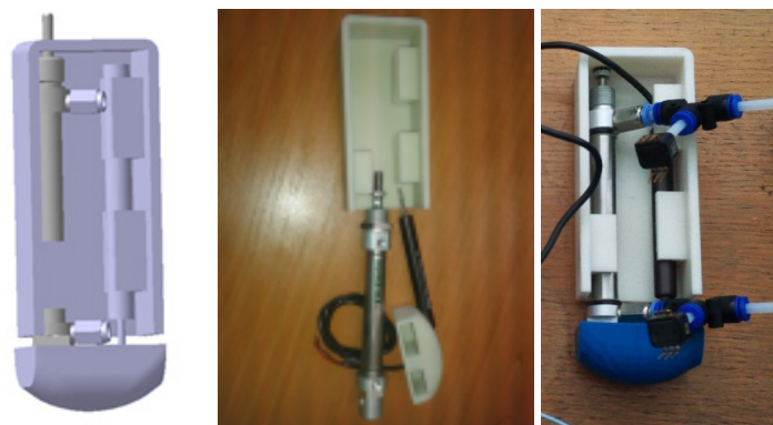
Figure 8. Haptic pneumatic probe (from the left to the right: CAD model, kit and assembled versions).
