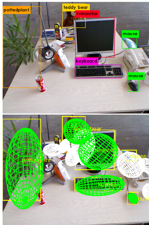
Figure 1: Our system is able to perform camera relocalization from objects detected in the image. Object detections (top) are modeled by ellipses, considered as projections of a known 3D scene model composed of 3D ellipsoids. The ellipsoids, once matched to 2D ellipses by our method, are reprojected in the image (bottom) using our estimated camera pose (green: inliers).
