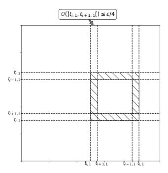
Figure 6: Example of bracket for d=2. With  $l=\mathbf{1}_{[t_{i+1,1};t_{j-1,1}]\times[t_{i+1,2};t_{j-1,2}]}$  and  $u=\mathbf{1}_{[t_{i,1};t_{j,1}]\times[t_{i,2};t_{j,2}]}$ , for any rectangle A,  $\mathbf{1}_A\in[l,u]$  if and only if its boundary  $\bar{A}\setminus\mathring{A}$  is included in the hatched area.
