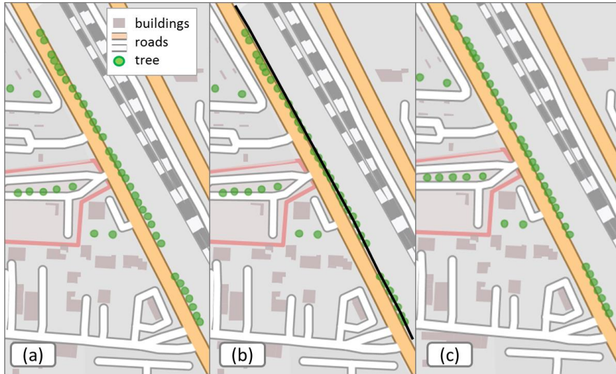
Fig. 6. a) Inaccurate trees overlapping a road. b) computation of an offset on the side of the road with trees. c) trees aligned on the offset line
