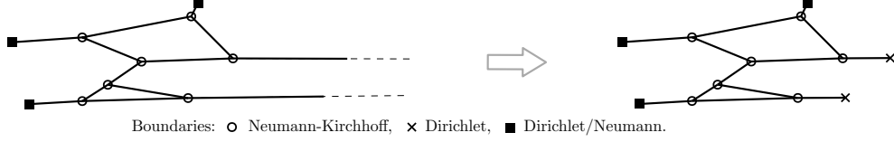
Figure 4. The figure represents an example of definition of the compact graph \tilde{\mathcal{G}}(\varphi) (on the right) from a specific infinite graph \mathcal{G}(\varphi) (on the left) composed by N_1 = 11 finite edges and \tilde{N}_1 = 2 infinite edges. We also underline the boundary conditions characterizing D(\tilde{A}) in \tilde{\mathcal{G}}(\varphi) .
