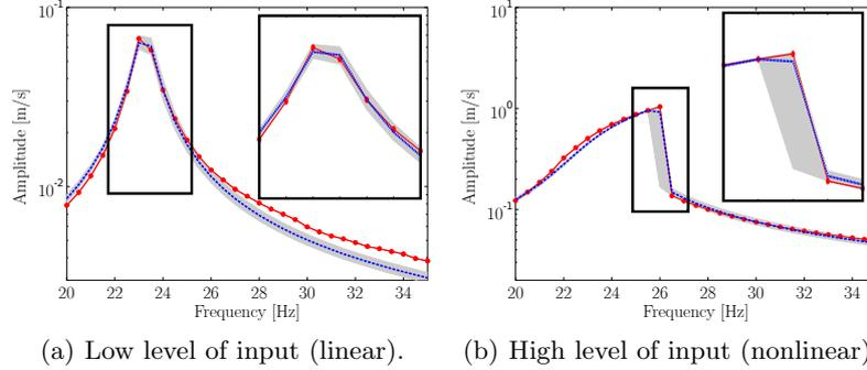
Fig. 6: Stepped sine curves comparison. The model mean is presented as  $-$ , the confidence band as gray fill, and the experimental realization as  $- \circ -$ .
