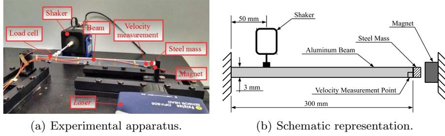
Fig. 1: Illustration of the experimental apparatus used.
