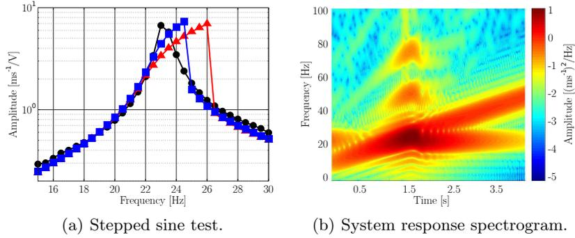
Fig. 2: Illustration of the system nonlinear behavior: (a) Stepped sine test for different levels of voltage applied in the shaker.  $\bullet$  - 0.01 V,  $\blacksquare$  - 0.10 V and  $\blacktriangle$  - 0.15 V; (b) Spectrogram of the system response.
