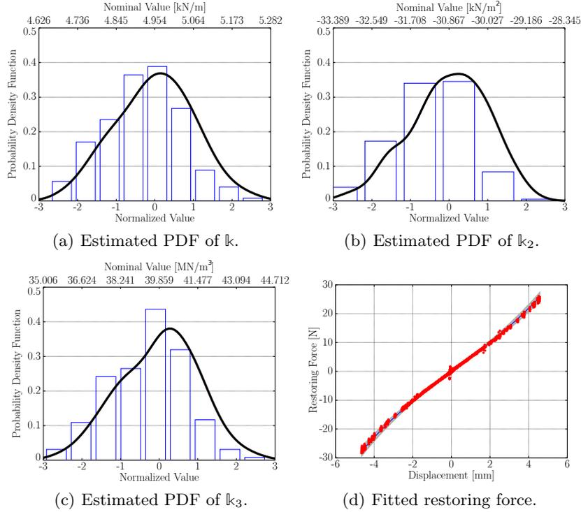
Fig. 4: PDFs for mechanical system stiffnesses and the fitted restoring force. (a, b and c) The PDF is represented by the solid line and the histogram by the bars; (d) The model mean is presented as —, the confidence band as grey shown, and the experimental realization as •.
