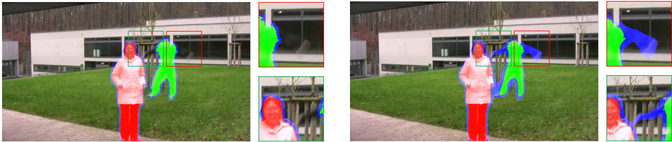
Fig. 3 Advantages of using the smart dilation mask, i.e. a smart border layer in the output map of our Multi-OSVOS network. (a) The border is obtained by simply dilating the output map of the network: some parts of the objects are not covered. (b) The border layer is learned by the network: the transition region is covered.
