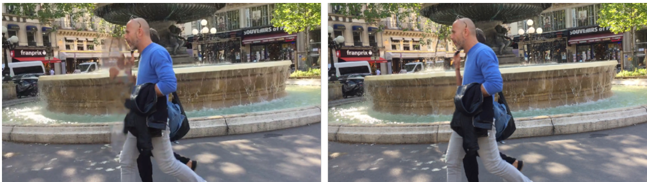
Fig. 14 The advantage of using the segmentation masks to separate background and foreground. Left: without separating background/foreground, the result have many artifacts. Right: the background and foreground are well reconstructed when being reconstructed independently.
