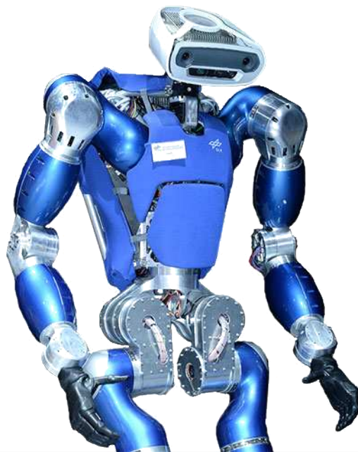
Fig. 1. Toro is a torque-controlled humanoid robot developed at DLR [3].
