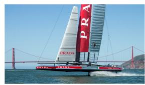
Fig. 1 - America's Cup catamaran propelled with two-element wingsail.
