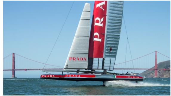
**Fig. 1 - America’s Cup catamaran propelled with two-element wingsail.**
