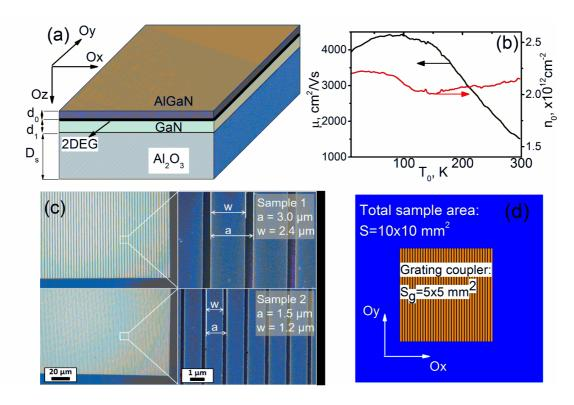
**Fig. 1.** (a) A schematic sketch of the bare AlGaN/GaN quantum well heterostructure. (b) Results of the measurements of temperature dependences of the mobility and the electron concentration of 2DEG. (c) Scanning electron microscopy (SEM) images of two plasmonic samples with different grating periods and strip width. (d) A sketch of the plasmonic sample with grating coupler.
