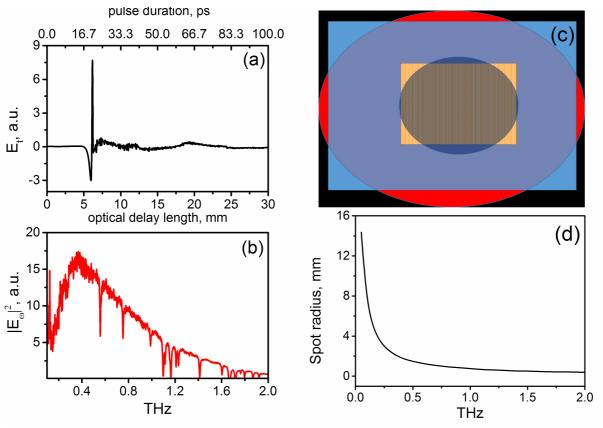
**Fig. 2.** (a) Waveform of the electric field of the THz pulse in the time-domain. (b) The corresponding power spectrum in the frequency-domain; (c) Sketch of the plasmonic sample illumination by different spectral harmonics. Wide red and narrow blue circles schematically illustrate the spot sizes corresponding to the lower and higher frequency harmonics, respectively. (d) Variation of the focal spot size with the frequency.
