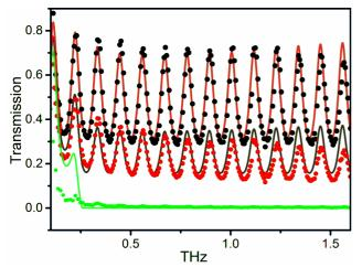
**Fig. 6.** Transmission spectra of Sample 2 for different polarization angles,  $\alpha = 0^{\circ}$ ,  $45^{\circ}$ , and  $90^{\circ}$  (black, red and green curves, respectively). Solid lines are the results of calculations according to Eq. (14). Circles are the results of the measurements.
