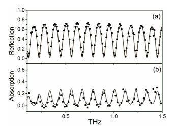
**Fig. 7.** Reflection (a) and absorption (b) spectra of Sample 2 for *p*-polarization. Solid lines are the results of calculations. Circles correspond to the measurements. Calculated absorption spectrum of the bare heterostructure is shown with the dash-dotted line.
