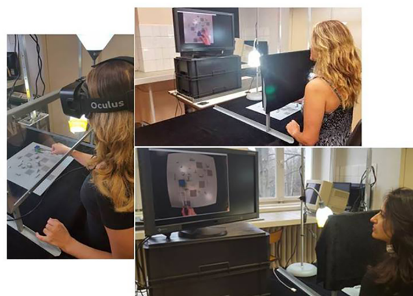
Fig 1. Snapshot views of the experimental platform. How individuals were seated, the two monitor positions (sideways and straight ahead), and examples of the 2D (top) and 2D fisheye (bottom) viewing conditions are shown. In the “natural” direct viewing condition, the subject was positioned as in the Oculus head-mounted virtual 3D stereo viewing scenario (left).
