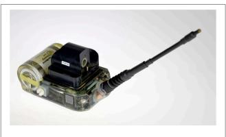
**FIGURE 2** | A CTD-SRDL tag, featuring a miniaturized CTD on top of the core unit, with the microcontroller below, the wet/dry sensor on the frontside, the battery on the rear, and the Argos antenna pointing forward.
