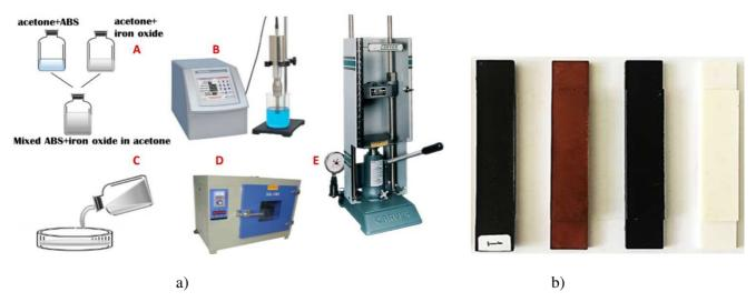
Figure 1. a) Fabrication process of the composites. b) Three groups of samples (from left to right): ferromagnetic composites, two conductive composites filled with copper and carbon black, and pure ABS.
