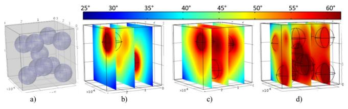
Figure 14. a) Microscopic scale of the ferromagnetic composite. Heat transfer of particles with b) 3% vol. fraction, c) 10% vol. fraction, and d) 17% vol. fraction.
