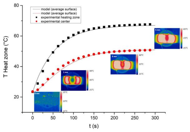
Figure 13. a) Theoretical and experimental temperatures as a function of time for the 17% vol. fraction composite.
