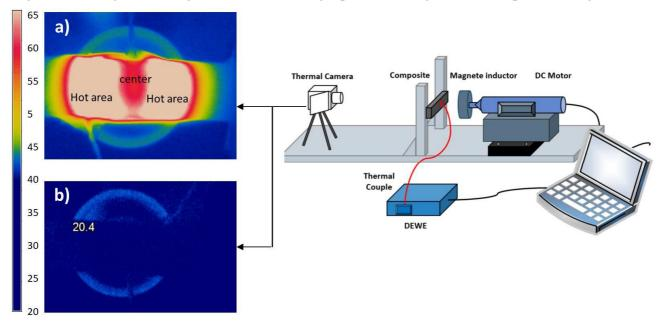
Figure 7. LFIH observation under 2.3 kHz AC magnetic field excitation. a) Ferromagnetic composite with 17% vol. of iron oxide. b) conductive composite with 15% of copper oxide.
