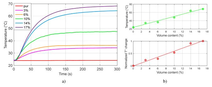
Figure 8. a) Evolution of the temperature with time at different particle fraction. b) Maximum temperature and normalized relative temperature change versus volume fraction concentration.
