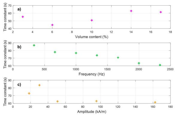
Figure 11. The time constant as a function of a) volume content, b) frequency of magnetic field, and c) amplitude of magnetic field.
