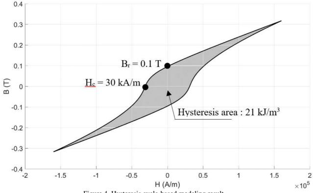
Figure 4. Hysteresis cycle-based modeling result.
