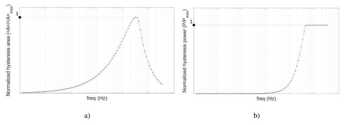
Figure 3. Logarithmic frequency dependence of a) normalized hysteresis area and b) normalized hysteresis power for a ferrite bulk (simulation result).
