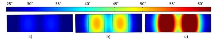
Figure 12. Spatial evolution of temperature for the macroscopic scale of the ferromagnetic composite with a) 3% vol. fraction, c) 10% vol. fraction and c) 17% vol. fraction.
