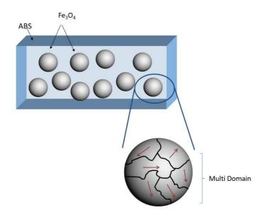
Figure 2. Schematic illustration of the magnetic composite.
