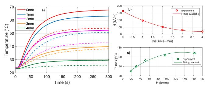
Figure 10. Time evolution of temperature at different distances between the composite and the magnetic inductor. Continuous lines show to the T<sup>o</sup> of hot source whereas dotted lines show the T<sup>o</sup> at the center. b) The amplitude of the magnetic field as a function of distance. c) Final temperature versus magnetic intensity.
