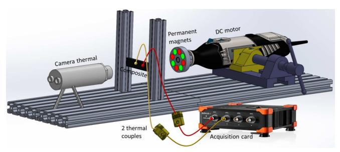
Figure 5. Experimental setup of the induction heating effect.
