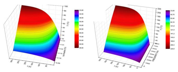
Figure 16. Performance of induction heating in terms of a) volume fraction and b) frequency of the magnetic field.
