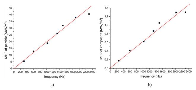
Figure 15. Magnetic heat power (MHP) versus frequency a) of  $Fe_3O_4$  particle and b) of composite doped with 17% vol.
