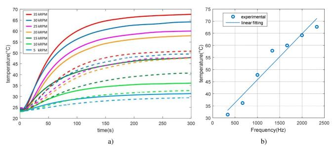
Figure 9. a) Temperature versus time at different motor speeds (kRPM). Continuous lines relate to the T° of hot source, whereas dotted lines referred to the T° at the center. b) Temperature versus frequency of alternative magnetic excitation.
