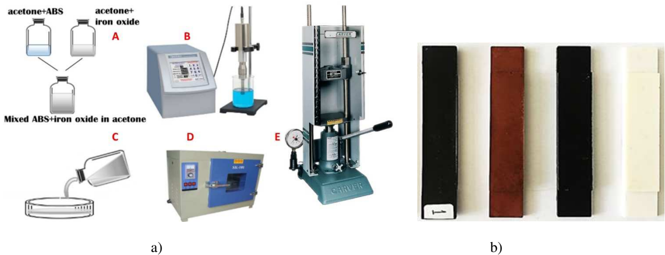
Figure 1. a) Fabrication process of the composites. b) Three groups of samples (from left to right): ferromagnetic composites, two conductive composites filled with copper and carbon black, and pure ABS.
