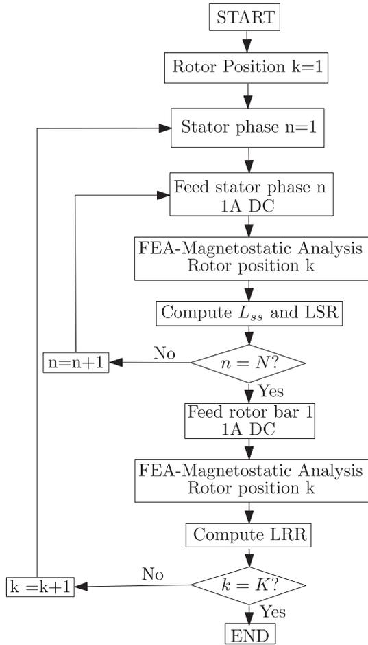
Fig. 4. Flowchart of inductance matrix computation of a faulty IM for each rotor position using FEA where  $N$  is the number of stator phases of the machine and  $K$  is the total of rotor positions to simulate.
