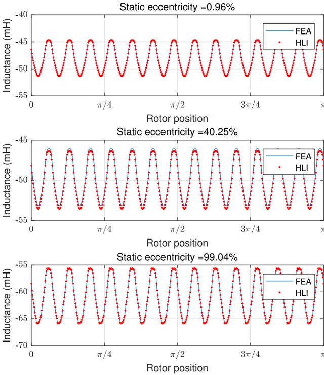
**Fig. 7.** Mutual inductance between the stator phase 1 and the stator phase 2 for three different levels of static eccentricity depending on the rotor position using FEA software and the proposed method (HLI).
