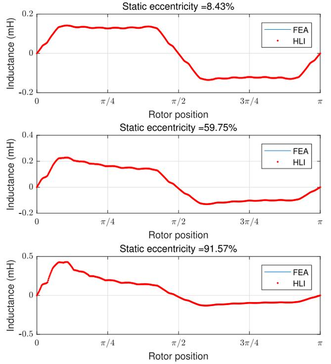
**Fig. 8.** Mutual inductance between the stator phase 1 and the rotor bar 2 for three different levels of static eccentricity depending on the rotor position using FEA software and the proposed method (HLI).
