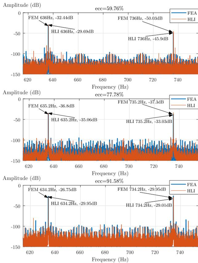
**Fig. 13.** Stator current spectrum obtained for three different levels of static eccentricity using FEA software and the proposed method (HLI) to compute the inductance matrix of the model. Besides, the frequency of the fault harmonic related components due to static eccentricity are highlighted for both the inductance matrix computed using FEA software and the proposed method (HLI).
