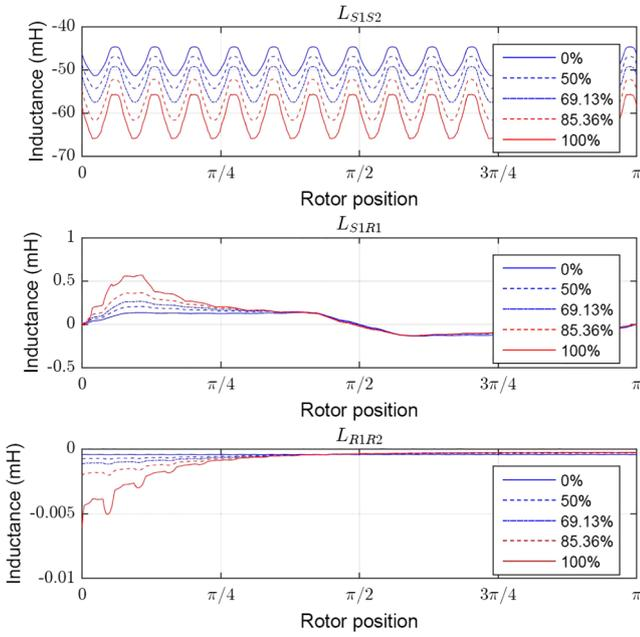
**Fig. 6.** Mutual inductance between the stator phase 1 and the stator phase 2 (top), between stator phase 1 and rotor bar 1 (middle) and between rotor bar 1 and rotor bar 2 (bottom) for 5 different degrees of static eccentricity (inside the levels 0–3 obtained with the GCL set) depending on the rotor position using FEA.
