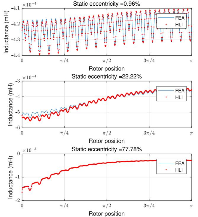
**Fig. 9.** Mutual inductance between the rotor bar 1 and the rotor bar 2 for three different levels of static eccentricity depending on the rotor position using FEA software and the proposed method (HLI).
