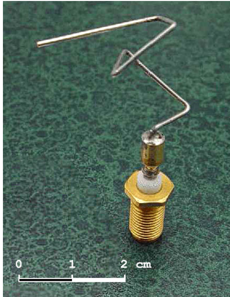
Figure 1: This unconventional antenna design was generated by NASA using evolutionary computation to optimize its radiation pattern [Hornby et al., 2006]. It was used in the ST5 spacecraft. (Image in the public domain.)
