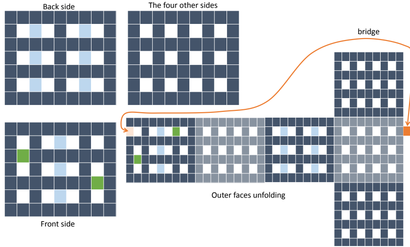
Fig. 5: The outer face unfolding in a cube unfolding fashion. The light-blue faces are used to link 2 lines, and the green faces are used to link 2 planes.
