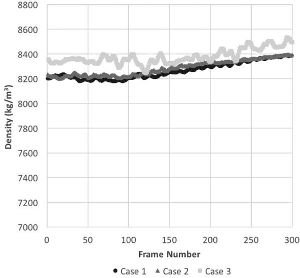
FIG. 6. Density results for three niobium samples.
