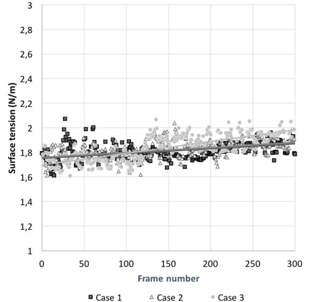
FIG. 5. Surface tension measurement for three niobium samples.
