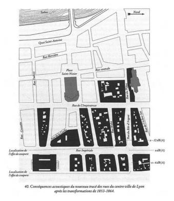
Figure 11.7 Acoustic consequences of the new layout of the streets in the centre of Lyon, after the transformations of 1853–64. Drawing by Olivier Balaÿ.
