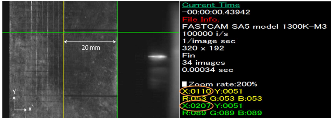
Fig.7 : Distance calibration in Photron software
