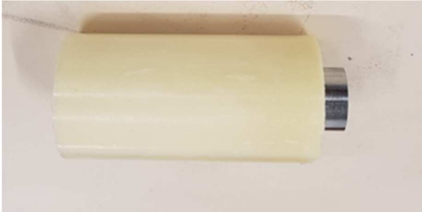
Fig.6 : Steel projectile inside foam housing
