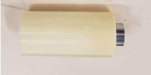
Fig.6 : Steel projectile inside foam housing
