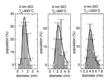
FIG. 3. Size distribution of the trilayer structures with a SiO layer thickness equal to 4 nm for annealing temperatures equal to 950, 990, and 1050  $^{\circ}$ C.
