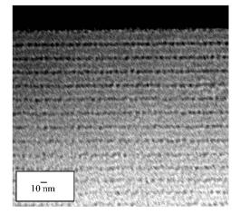
FIG. 2. Cross-section view of a multilayer with a SiO layer thickness equal to 3 nm and annealed at 1050  $^\circ\text{C}.$
