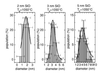
FIG. 4. Size distribution of the trilayers annealed at 1050 °C with SiO layer thicknesses equal to 2, 3, and 5 nm.
