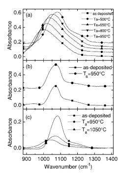
FIG. 1. Infrared absorption spectra from (a) a single 200 nm SiO layer, (b) a single 200 nm SiO<sub>2</sub> layer, and (c) the active layer of the SiO/SiO<sub>2</sub> multilayers, for the as-deposited samples and for the samples annealed at the temperature  $T_a$ .
