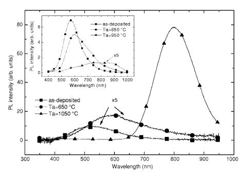
FIG. 5. Photoluminescence spectra of a multilayer with a 3 nm SiO layer thickness annealed at different temperatures. The inset represents the PL spectra for the single SiO layer.
