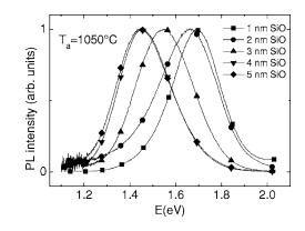
FIG. 6. Normalized PL spectra of multilayers annealed at 1050 °C for different SiO layer thicknesses.
