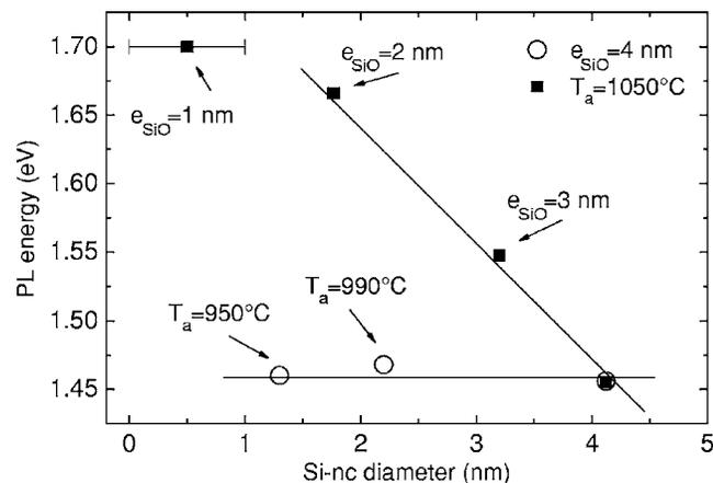
FIG. 7. PL energy of the multilayers as a function of the nc-Si diameter for  $T_a$  equal to 1050 °C (full squares). The empty circles represent the PL energy of the multilayer with a SiO thickness equal to 4 nm, for different annealing temperatures. The lines are guides for the eyes.
