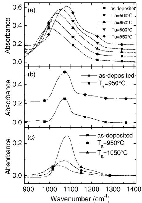
FIG. 1. Infrared absorption spectra from (a) a single 200 nm SiO layer, (b) a single 200 nm SiO<sub>2</sub> layer, and (c) the active layer of the SiO/SiO<sub>2</sub> multilayers, for the as-deposited samples and for the samples annealed at the temperature *T<sub>a</sub>*.
